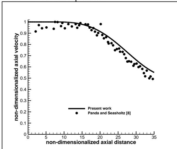
Figure 3. Centerline velocity with exit Mach of 1.4 versus axial distance.
