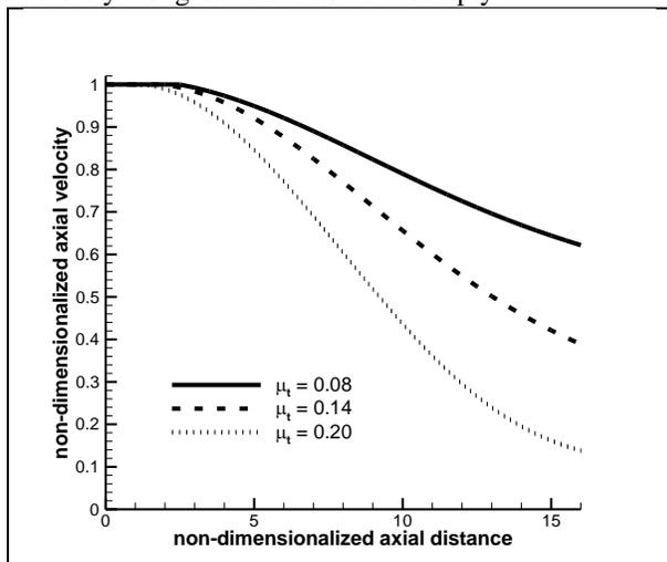
Figure 4. Centerline velocity vs. axial distance at different turbulent eddy viscosities.
