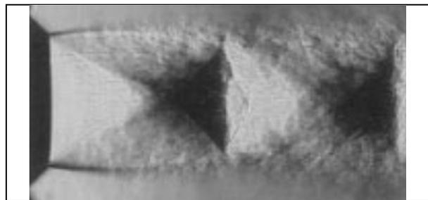
Figure 1- Schlieren image of an under expanded jet at Mach number of 1.42 [1].
