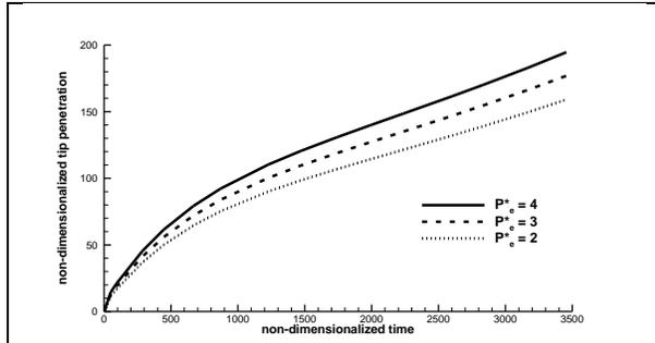
Figure 7 Tip penetration length versus time for different pressure ratios.
