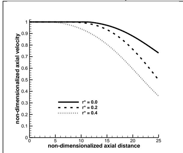
Figure 5. Variation of axial velocity versus axial distances at different radial positions.
